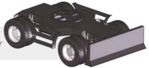
Undercarriage with front dozer blade
