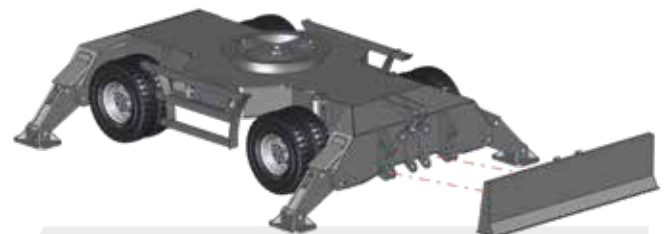
3000 mm wide HD-undercarriage with front and rear outriggers (front blade optional)
